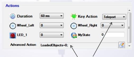
You now need to set the key action to "Teleport" and also set the LoadedObjects = 0 to clear the loaded object counter at the stage of teleporting
